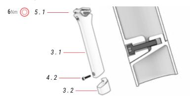
▲ Bolt 4.2 must be inside the seat post and parts 3.1 and 3.2 aligned.
