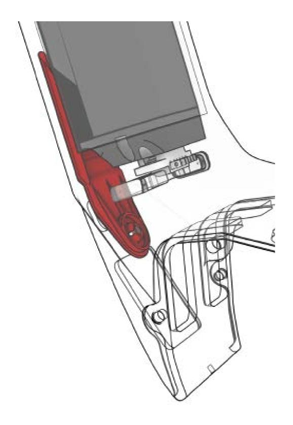
**ASSEMBLY:** REMOVE THE PLASTIC FILM PROTECTING THE GLUE ON THE PART. THEN, INSERT IT INTO THE DIAGONAL TUBE OF THE BIKE AND ASSEMBLE IT BY PRESSING IT AGAINST THE HOUSING OF THE SCREW (MARKED IN RED) THAT FIXES THE MOTOR COVER. FINALLY, PRESS THE PART AGAINST THE FRAME SO THAT THE GLUE FIXES IT COMPLETELY.
