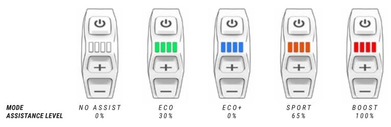
In order to increase the life of the battery and prevent a full discharge which may damage it, the assistance modes are limited based on the state of charge of the battery:
