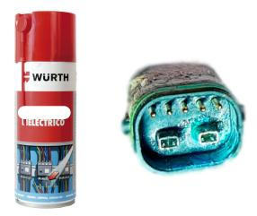
When electrical connections come into contact with damp spots or are clogged due to external contamination, a chemical reaction occurs, causing a build-up of lead sulphate crystals in the connections. In other words, the copper on the contacts will rust, resulting in conductivity problems.
