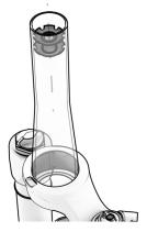
⚠ It is recommended to use a duller to ensure that the spider is inserted into the steerer tube perfectly aligned.
