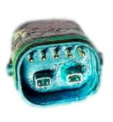
When electrical connections come into contact with damp spots or are clogged due to external contamination, a chemical reaction occurs, causing a build-up of lead sulphate crystals in the connections. In other words, the copper on the contacts will rust, resulting in conductivity problems.
