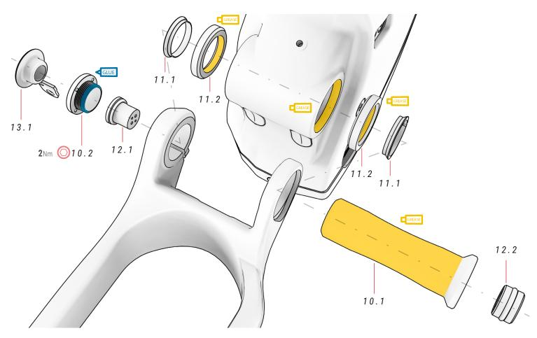
The maximum tightening torque of part 10.2 is 2 Nm, since it is designed to prevent gaps. Bolt 12.2 will secure part 10.2 and the remaining swingarm assembly.
