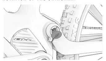
3. ALWAYS CONNECT THE BATTERY CHARGER FIRST AND THEN REMOVE THE PLUG FROM THE POWER SOCKET.
