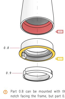
Part 0.8 can be mounted with the notch facing the frame, but part 0.9 must always be mounted in the first position, as shown in the images.
