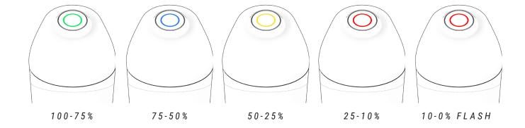
In models equipped with the Core display, the XPRO DD battery charge level will be shown with the ring of LEDs. The capacity of the XPRO DD battery will be added to the capacity of the bicycle's internal battery and the display will show the total charge of both batteries as follows:
