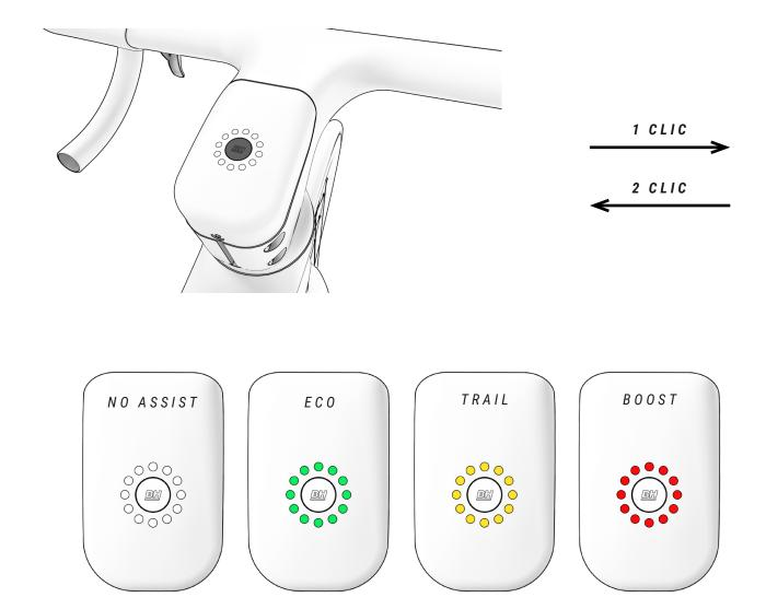
In order to increase the life of the battery and prevent a full discharge which may damage it, the assistance modes are limited based on the state of charge of the battery:
